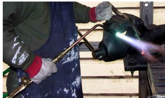
Oxy-acetylene gas welding
