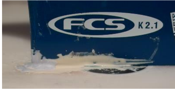
Surf board fin repaired with epoxy resin
